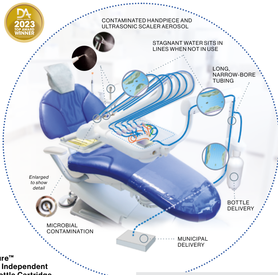
Stages of microbial growth in untreated waterlines
