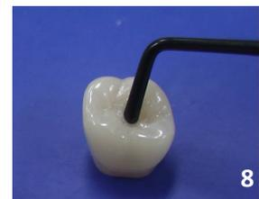
The photos below show the conditions of the paste after being used to fill a SUS jig and compressed with a SUS rod at a load of 2 kgf. The photos show that Estelite Posterior paste tends to resist seeping around the filling instrument.
