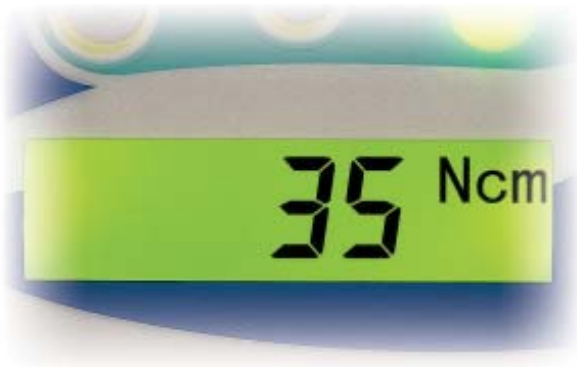
Torque control – adjustable from 5 to 50 Ncm.
