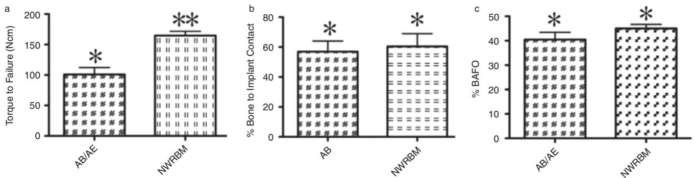
Fig. 2. (a) Significantly higher removal torque ( $P = 0.01$ ) was observed for the NWRBM surface compared with the AB/AE, whereas (b) BIC and (c) BAFO ( $P > 0.35$  and  $P > 0.11$ , respectively) statistics summary (mean  $\pm$  95% confidence intervals) presented no significant differences.
