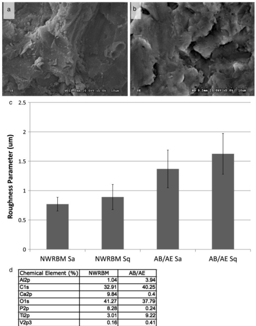
Fig. 1. Scanning electron micrographs of the (a) NWRBM surface depicting evidence of blasting particles, and (b) AB/AE. (c) Measurable roughness parameters ( $S_a$  and  $S_q$ ) showed overall higher roughness profile for the AB/AE group compared with the NWRBM ( $P < 0.001$ ). (d) Average chemical composition for the different surfaces as observed in the XPS spectra.
