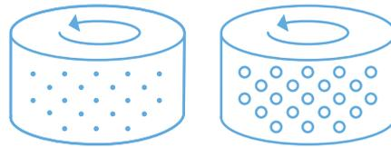
TOKUYAMA DENTAL produces OMNICHROMA fillers based on its own patented “*Sub-Micro-Pearl-Technology*”. In this process, the Sol-Gel method is used to progressively coat spherical fillers in an organic solution. After several weeks, the fillers have “grown” evenly in a spherical shape and are exactly 0.26  $\mu\text{m}$  in size. In this optimal size, the desired colour adaptation effect is achieved precisely in combination with other outstanding physical properties.
