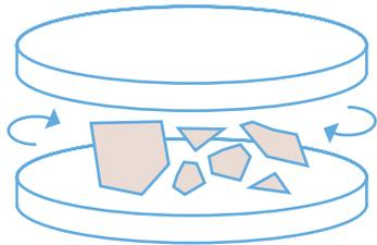
Glass materials are ground until the individual filler particles are within a desired size range. However, an exact control is not possible in this way, so that the filler particles differ significantly in shape and size. This becomes particularly clear as soon as the fillers in question are observed under the scanning electron microscope.
