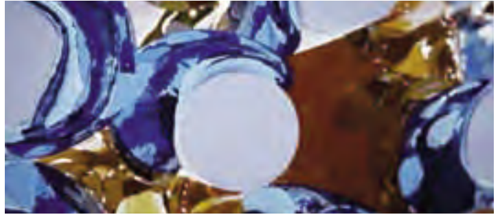
Inside everStick fibre. Individual fibres, bis-GMA and PMMA for the unique IPN structure.
