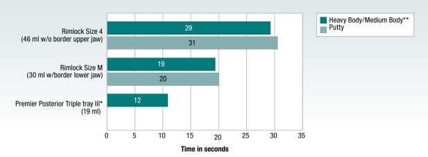
Fig. 8: Required time (in seconds) to fill different tray types from the Pentamix" Lite Automatic Mixing Unit with either a heavy body or putty impression material.
